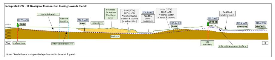
Figure 6-21 - Northwest - Southeast cross-section showing Conceptual Hydrogeological Model for the Site (2023)
