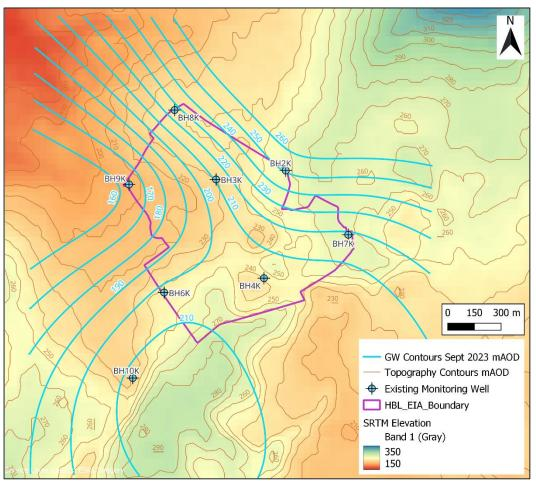
Figure 6-16 - Groundwater Contours September 2023 with Topography
