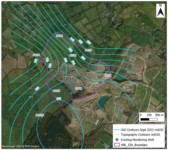
Figure 6-15 - Groundwater Contours September 2023 with aerial and Topography
