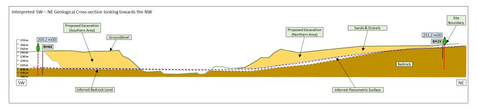
Figure 6-20 - Southwest – Northeast cross-section showing Conceptual Hydrogeological Model for the Site (2023)
